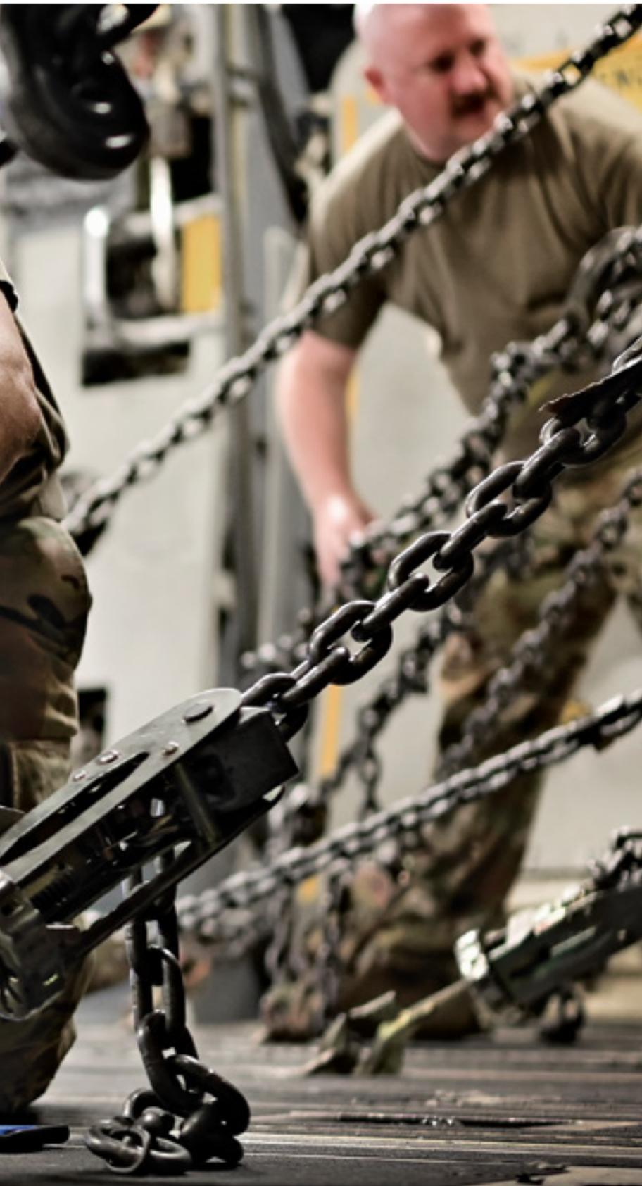
A U.S. Air Force C-17A Globemaster III aircraft loadmaster measures the restraints on a U.S. Army M1A2 Abrams Main Battle Tank at Ali Al-Salem Air Base, Kuwait. (U.S. Air Force photo)
