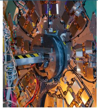
Muon Resistive Plate Chamber in the PHENIX detector at Brookhaven National Laboratory's Relativistic Heavy Ion Collider.
